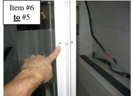
Tighten screws holding **Rear Doorframe** to **Center Divider**
